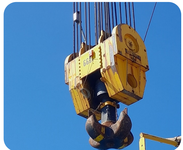
2500T Crane - Hoist Wire MRT Inspection
