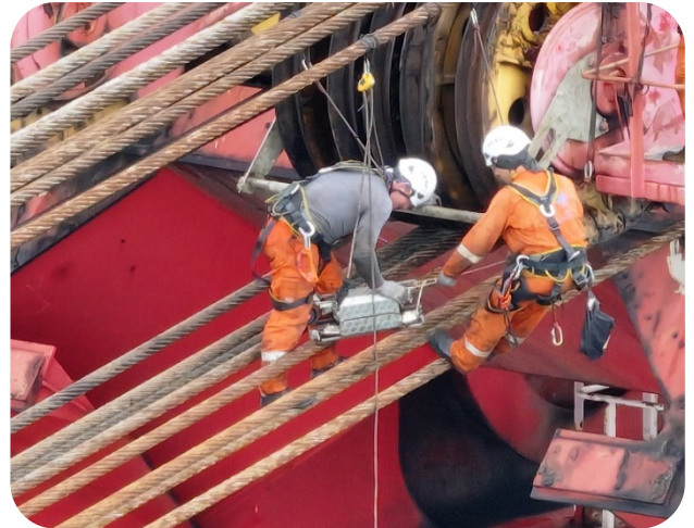
12000T Crane - Boom Wire MRT Inspection
