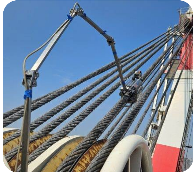
4000T Crane - Boom Wire MRT Inspection
