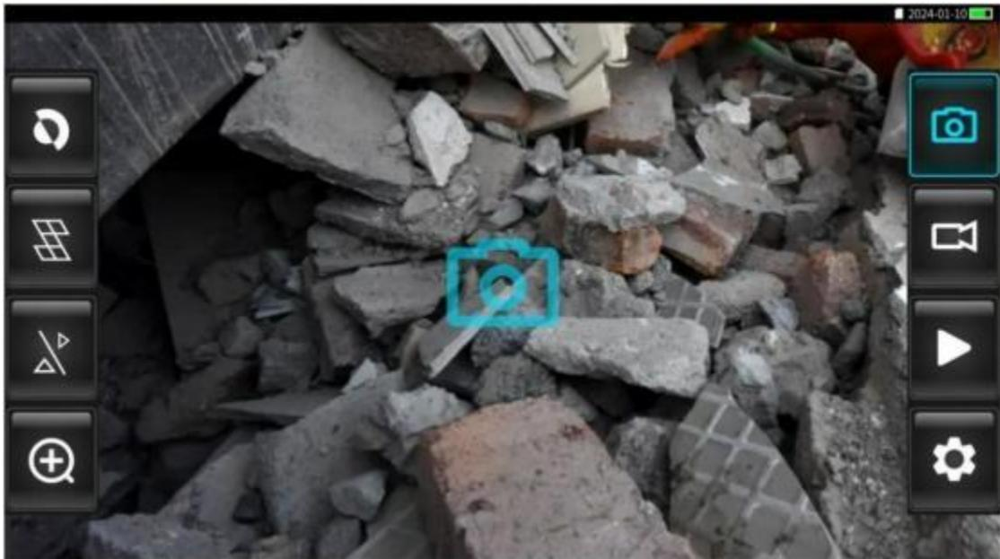
**Recording:** Click the icon
